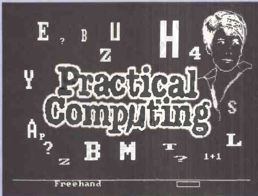
Input to the Pencept Penpad is analysed letter-by-letter by the host computer, which reproduces it in one of several standard sizes. It also accepts freehand input and provides graphics facilities such as circle drawing and colour infill.
